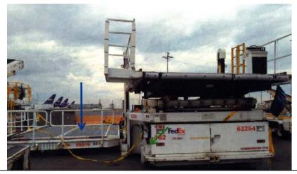
Photo 1 of 1 – Photos shows a view of the Commander 30H Cargo Loader with auxiliary deck attached. The blue arrow is indicating the auxiliary deck that struck the victim. The e-stop pendent box is indicated by the green arrow. The operator controls are located in the upper right side of the photo.
