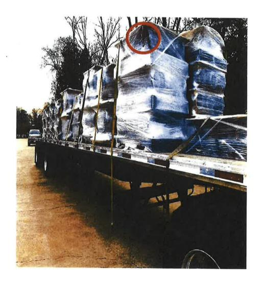
Photo demonstrates the scene on the day of the accident. The employee fell off the left side of the trailer. The red circle indicates the strap that is hung onto the top of the pallet stack.
