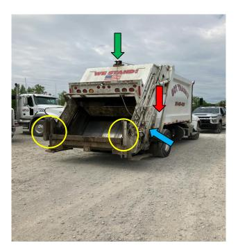
The photo shows the Kenworth #22, rear loading garbage truck involved in the accident. The red arrow indicates the approximate area where the victim was struck and pinned by the dumpster. The green arrow shows the cable/winch system that was used to lift and empty the dumpster. The yellow circles show the location of the locking mechanisms that lock the dumpster in place before the lifting process is performed. The blue arrow shows the location of the manual controls.
